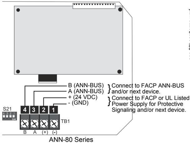
**Figure 3 Wiring the ANN-80 Series to an FACP**
