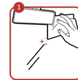
Clean the windshield and paste the electrostatic film onto it. Avoid introducing air bubble. DO NOT paste the film repeatedly.
