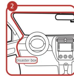
Paste the device onto the electrostatic film and route cable to the disaster box for power supply.
