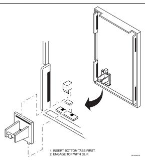
Figure 1. Tamper Magnet Installation
