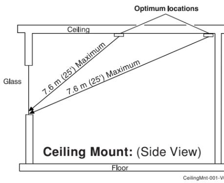
**NOTE:** If the device is ceiling mounted, the end with the hole (Microphone end) should face the protected glass.
