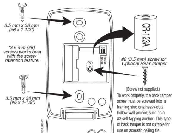
\*The screw retention feature simplifies installation: A rib in the screw cavity lightly holds the screw in place when installing the detector.
